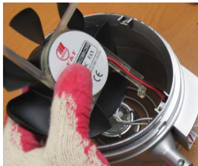
STEP 7. Mount new motor by inserting wires through the hole first
