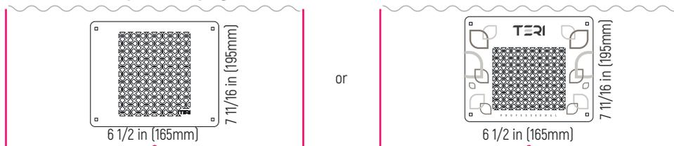
1. Cut a 165x195mm hole in the table, according to the diagram. We recommend placing the hole in front of the manicure master, depending on the model of the table and the number and sizes of cabinets.
